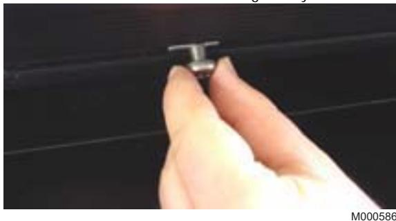
7. Put the lower horizontal housing in place by interlocking the notches in the screws.
